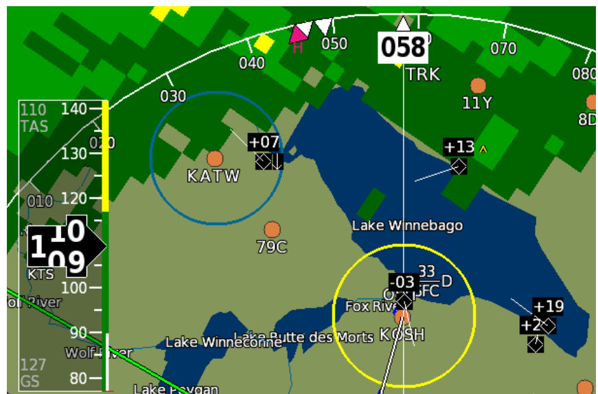
Traffic as it appears on the moving map screen. The digital value indicates the difference in altitude from your airplane in hundreds of feet. The line segment indicates the direction of travel of the traffic.
