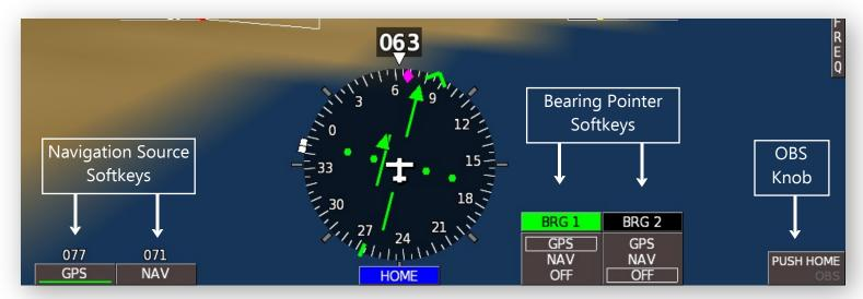
The **BRG softkeys** display GPS and VOR/LOC (NAV) choices based on installed navigation equipment. The bearing pointers simply point to the selected navaid or waypoint programmed into the navigation equipment. BRG 1 is a single shafted arrow and BRG 2 is displayed as a double-shafted arrow. Primary VOR/LOC (NAV1)
