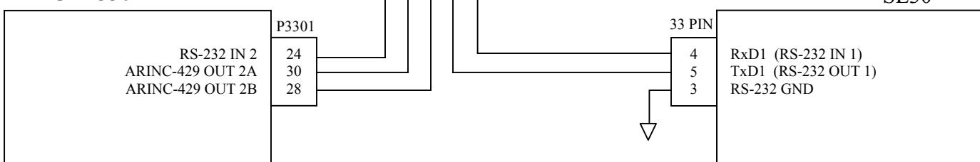
NOTE 1 : These connections are for redundancy in case of loss of MFD 1, normally supplied from inter display communications.
