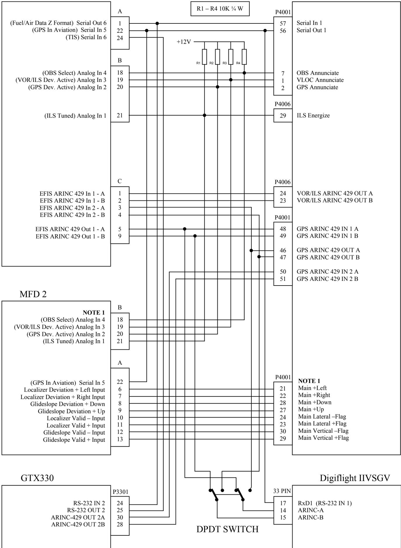
NOTE 1 : These connections are for redundancy in case of loss of MFD 1, normally supplied from inter-display communications.
