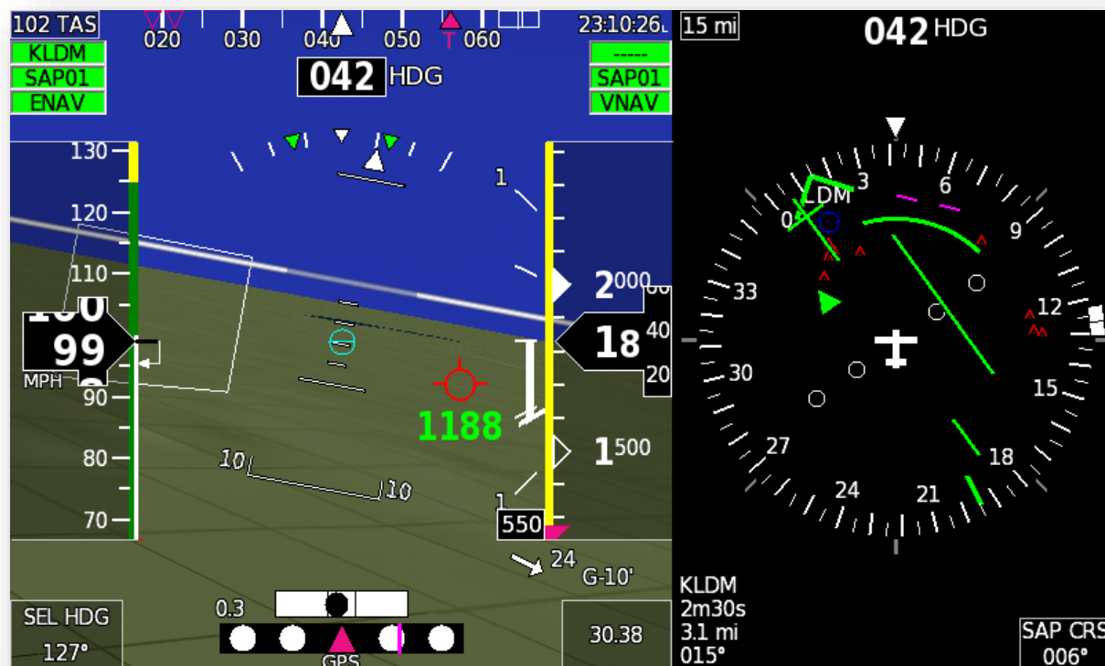
PFD HSI page showing the correlation between the Course Deviation Bar position and the Synthetic Approach final approach course Highway-In-The-Sky (HITS) boxes.
