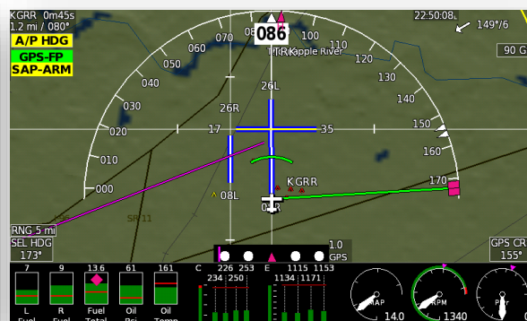
Arc View with engine strip and airspeed/altimeter tapes off.
