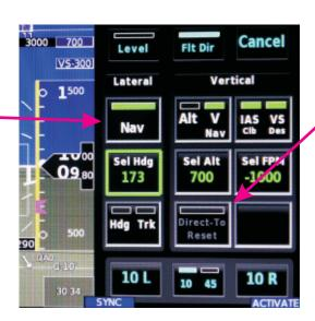
When the EFIS navigation mode is the internal GPS flight plan, Direct-To Reset will reset the flight plan origin to the present position. This allows going direct to the the next waypoint easily.
