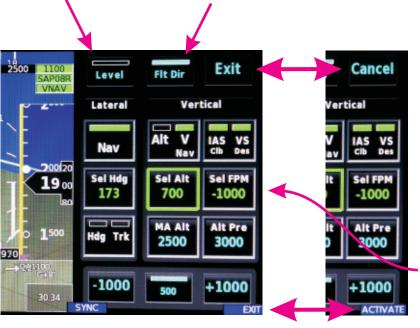
Exit - No changes to autopilot modes/targets are pending. Pressing this exits the A/P mode control panel.
