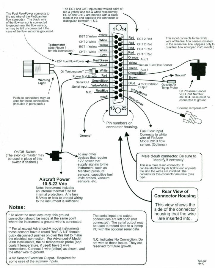
Figure 5 -- Connector A Wiring - Model 2000 for 4-Stroke Engines
