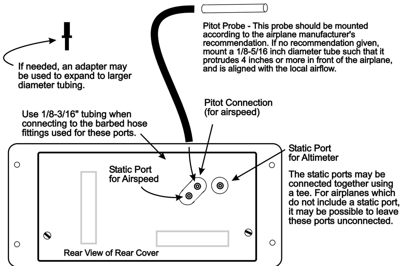
The altimeter/VSI and airspeed sensing is made by measuring the pitot and static air pressures. The altimeter/VSI requires only the static pressure, while the airspeed requires both pitot and static air pressures.
