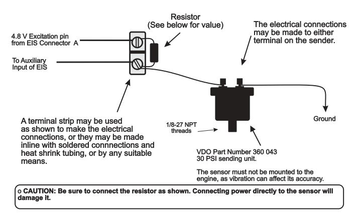
The sender may be set up to operate accurately over any of 4 different scales. For normally aspirated engines either the 0-5 or 0-10 psi range is typically used. For fuel injected engines normally the 0-28 psi range is used.
